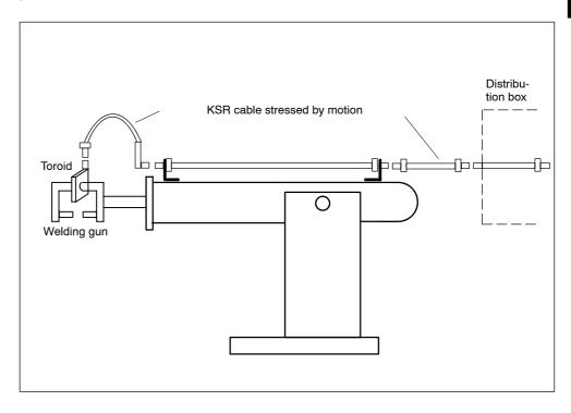
If the cable is divided into several segments, shielding connections must be made as shown in the following figure.
