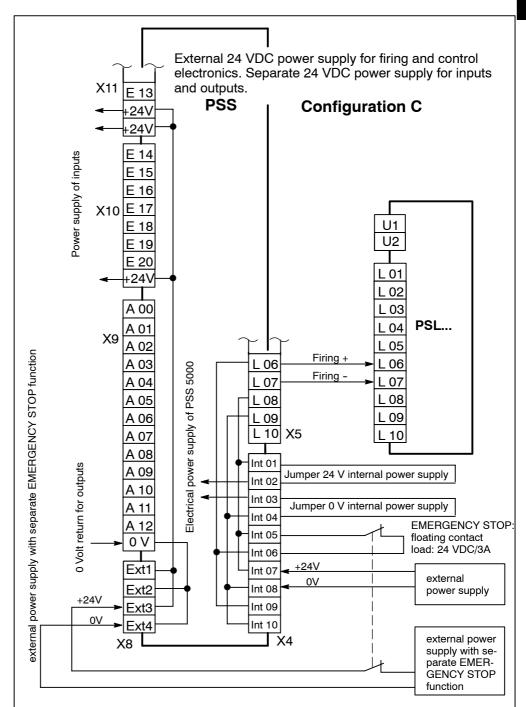
When using an **external power supply** for **inputs and outputs**, according to configuration D, the **floating contact** connected to Int 05 – 06 will interrupt only the **firing**. Additional provisions must be made to secure the **E-Stop function** for the **inputs and outputs**, using an **external auxiliary E-Stop contact** in the feeder line to the external power supply.
