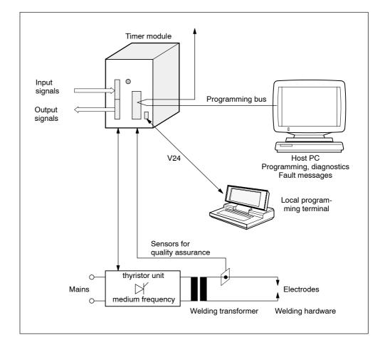
The welding timers are equipped with microprocessors. Up to **256** welding programs can be programmed and called up. Single spot (SING), repeat mode (REPT) or seam operation can be selected.
