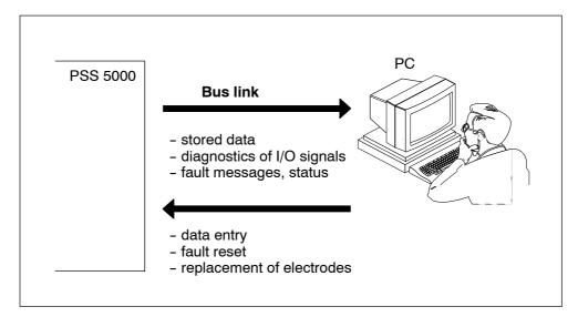
On the front panel of the timer is a V24 interface. This can be used for connecting a laptop for example. This laptop can be used for programming as well as to operate the timer on location.
